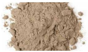
Bentonite is a very widely distributed clay material that is the result of the devitrification and chemical alteration of glassy volcanic ash or tuff. Bentonite should be used as the name of a rock derived from volcanic glass and it is commonly composed of the mineral montmorillonite but less often of beidellite.
